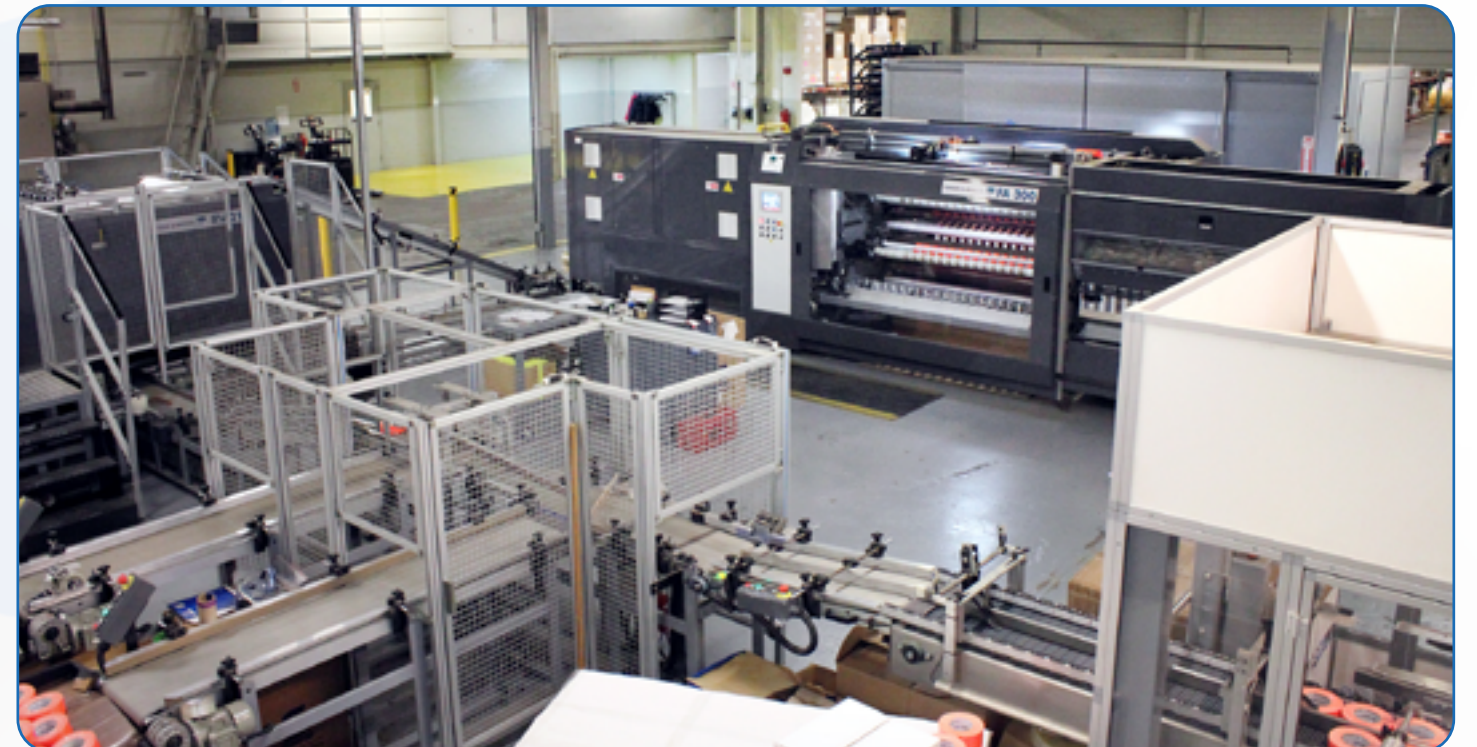
Photo: Wide web jumbo roll processing with integrated open core in-line roll wrapping and automated packaging.
