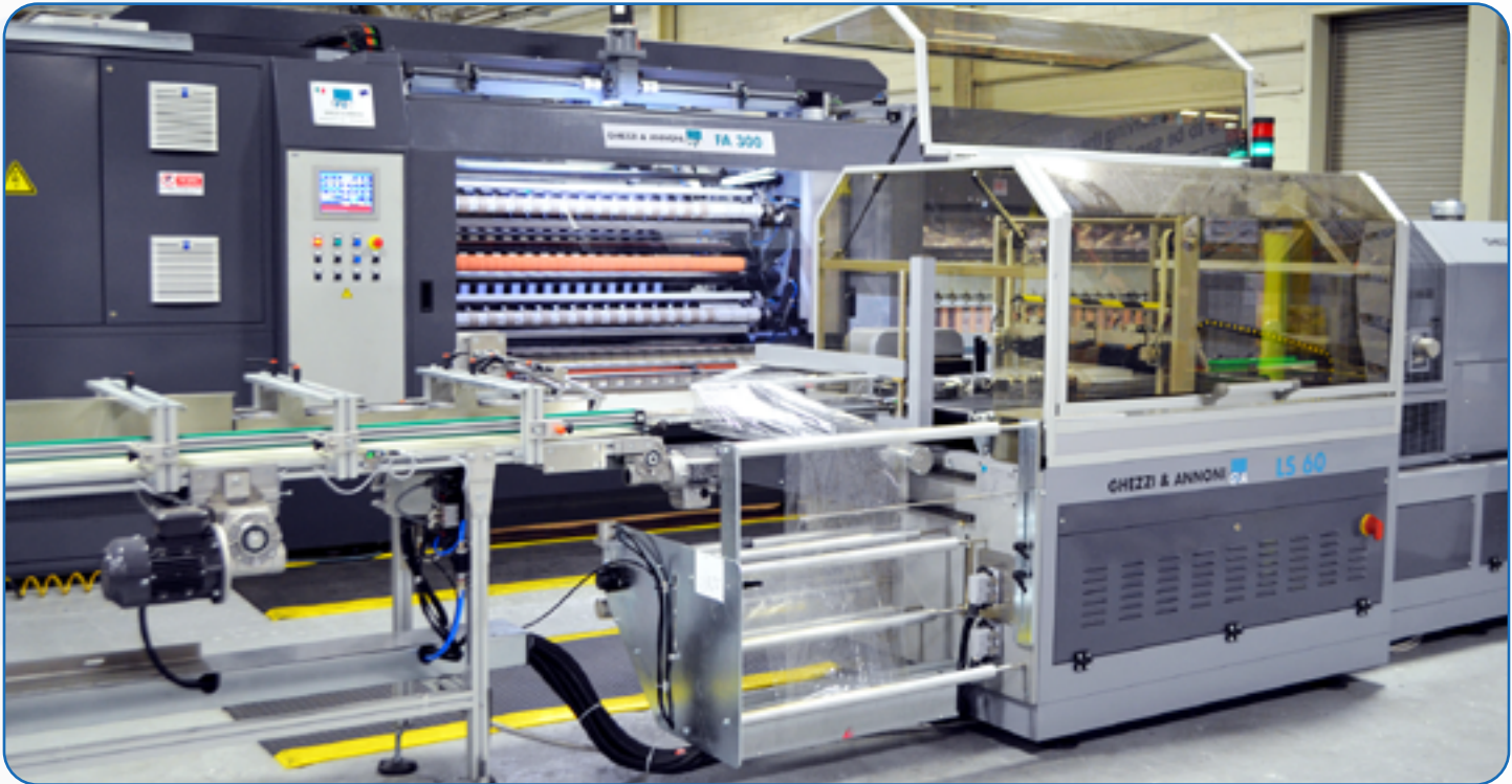
Photo: Wide web jumbo roll processing with integrated closed core in-line roll wrapping and multi-roll wrap options available.
